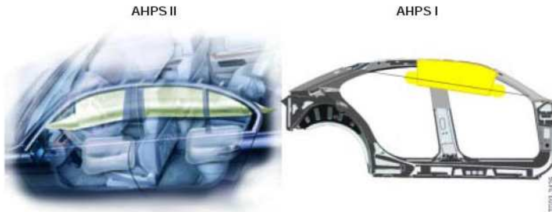
Fig. 20: Identifying AHPS II And AHPS I Part Courtesy of BMW OF NORTH AMERICA, INC.
