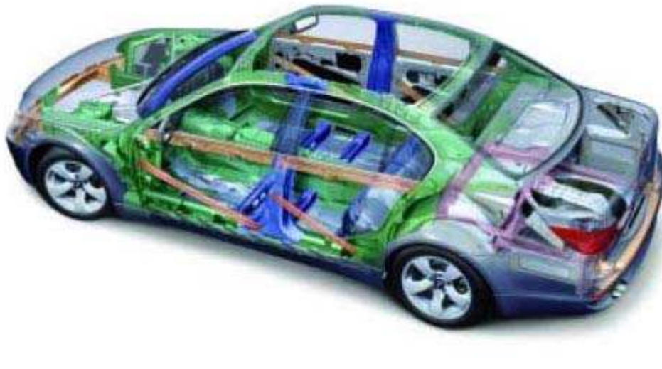
Fig. 7: Identifying Passenger Safety Cell E60 And Energy Absorbing Body Structures System Courtesy of BMW OF NORTH AMERICA, INC.
