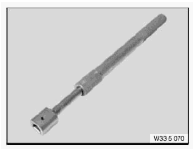
Fig. 43: Extension Piece (2) (33 5 070) Courtesy of BMW OF NORTH AMERICA, INC.
