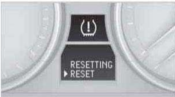
Fig. 25: Tire Pressure Monitor Status Display Courtesy of BMW OF NORTH AMERICA, INC.
