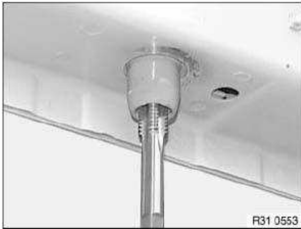
Fig. 8: Creating Locating Thread For Helicoil Thread Insert Courtesy of BMW OF NORTH AMERICA, INC.
