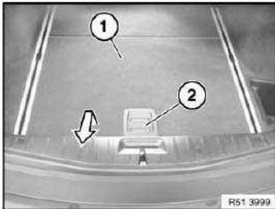
Fig. 502: Luggage Compartment Floor Trim Panel And Handle Courtesy of BMW OF NORTH AMERICA, INC.
