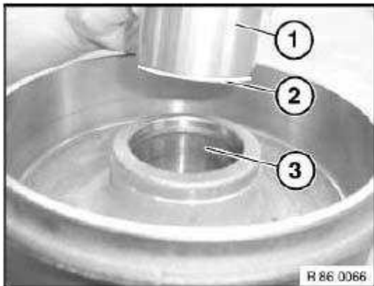
Fig. 103: Identifying Wheel Bearing, Lathe-Turned End & Center Of Bore In Brake Drum Courtesy of BMW OF NORTH AMERICA, INC.
