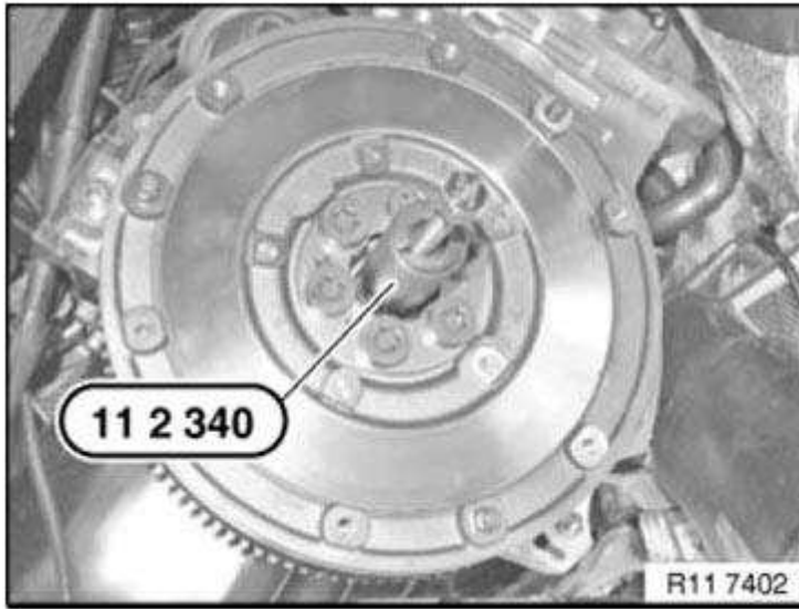
Fig. 157: Removing Guide Bearing Using Special Tool 11 2 340 Courtesy of BMW OF NORTH AMERICA, INC.
