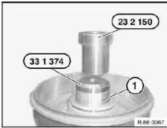
Fig. 104: Identifying Wheel Bearing With Special Tool (23 2 150 & 33 1 374) Courtesy of BMW OF NORTH AMERICA, INC.
