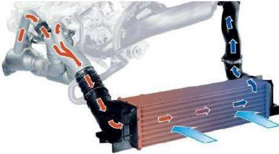
Fig. 42: Identifying Charge-Air Cooling Operations Diagram Courtesy of BMW OF NORTH AMERICA, INC.
