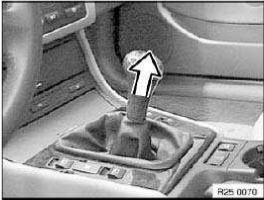
Fig. 18: Detaching Knob With Firm Tug Courtesy of BMW OF NORTH AMERICA, INC.
