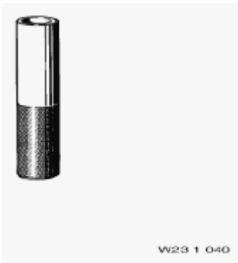
Fig. 27: Drift (23 1 040) Courtesy of BMW OF NORTH AMERICA, INC.
