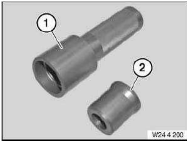
Fig. 61: Drift And Slip Bush (24 4 200)
