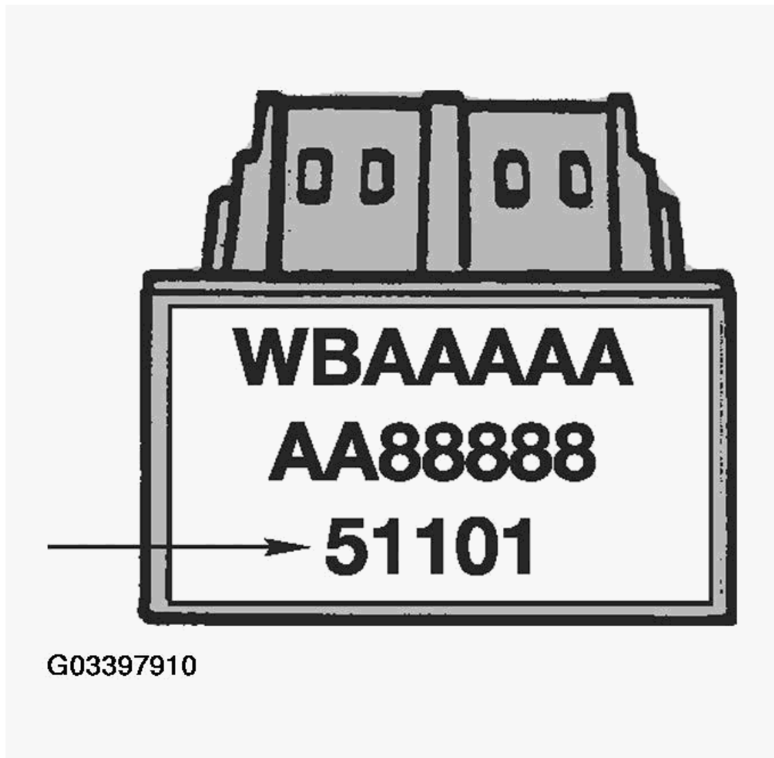
Fig. 56: Identifying Coding Plug Identification Number Courtesy of BMW OF NORTH AMERICA, INC.
