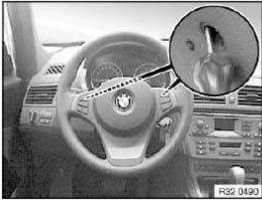
Fig. 82: Inserting Torx Screwdriver (T30) Horizontally Into Opening On Reverse Side Of Steering Wheel Courtesy of BMW OF NORTH AMERICA, INC.
