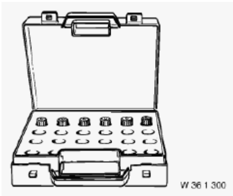
Fig. 9: Set Of Wheel Stud Adapters (36 1 300) Courtesy of BMW OF NORTH AMERICA, INC.
