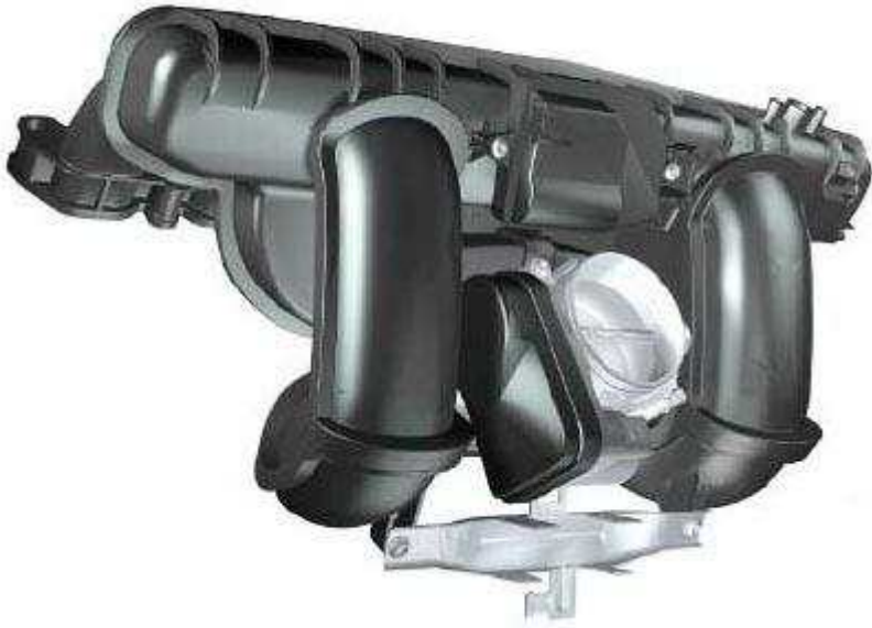
Fig. 20: Identifying 3-Stage DISA Intake Manifold Courtesy of BMW OF NORTH AMERICA, INC.
