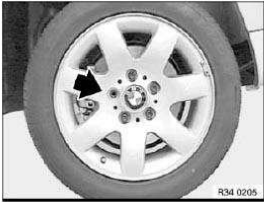
Fig. 12: Locating Wheel Stud On Each Rear Wheel Courtesy of BMW OF NORTH AMERICA, INC.
