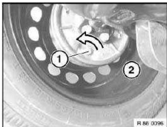
Fig. 11: Identifying Adjusting Screw & Road Wheel Courtesy of BMW OF NORTH AMERICA, INC.
