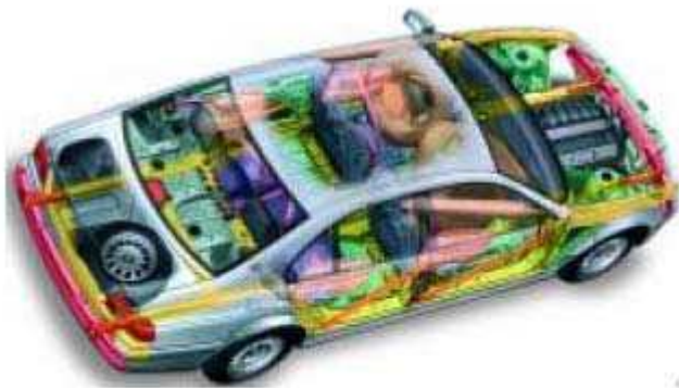
Fig. 2: Identifying Multiple Restraint (MRS) System Courtesy of BMW OF NORTH AMERICA, INC.
