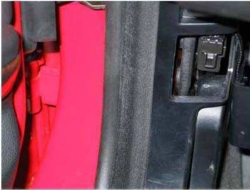
Fig. 22: Position DLC For 3 Series Models And Opened Design Cover / Closed Functional Cover Courtesy of BMW OF NORTH AMERICA, INC.
