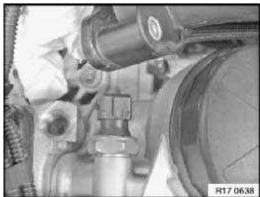
Fig. 61: Locating Mount Oil Pressure Switch On Filter Housing Courtesy of BMW OF NORTH AMERICA, INC.
