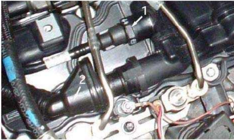
Fig. 28: Identifying Charge Air Suction Pipe Courtesy of BMW OF NORTH AMERICA, INC.
