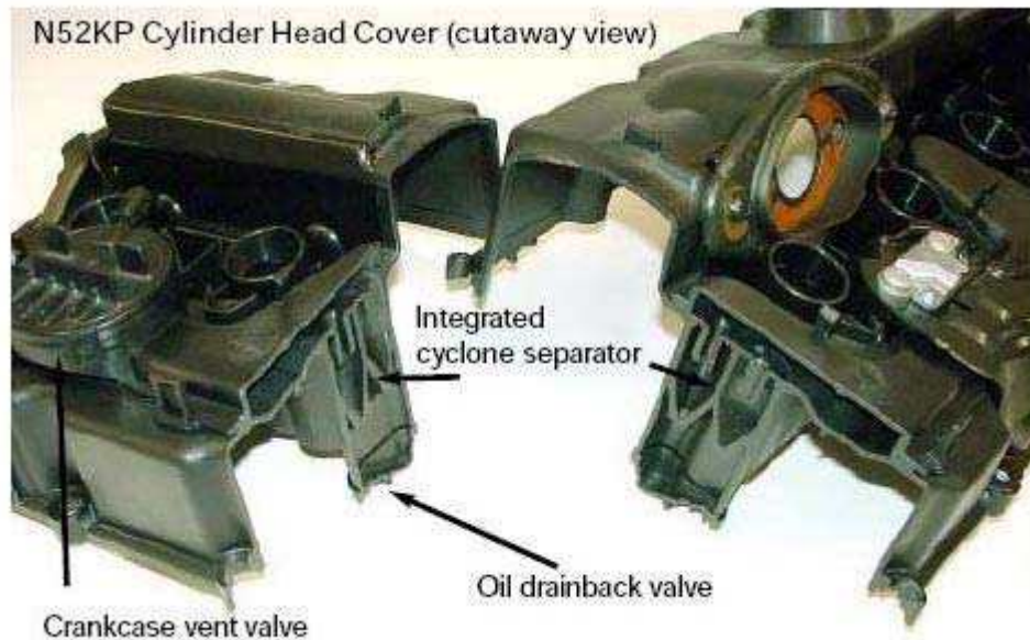
Fig. 23: Cylinder Head Cover Components Location Courtesy of BMW OF NORTH AMERICA, INC.
