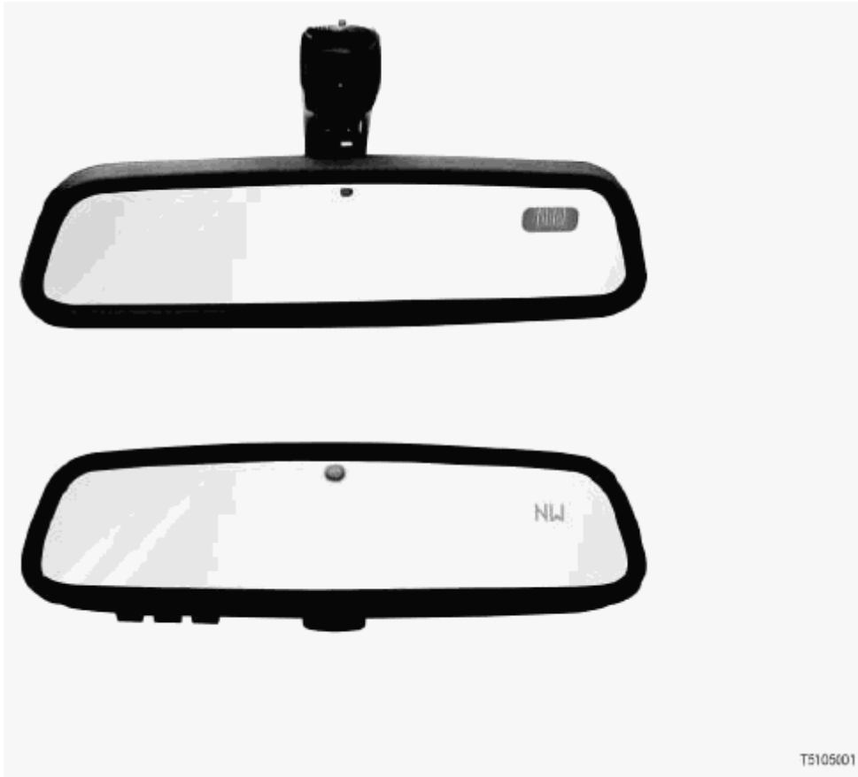
Fig. 1: Interior Mirror With Digital Compass Courtesy of BMW OF NORTH AMERICA, INC.
