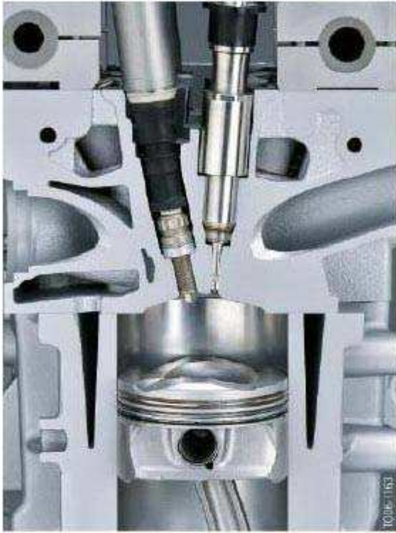
Fig. 14: Identifying Fuel Injector In Combustion Chamber Courtesy of BMW OF NORTH AMERICA, INC.
