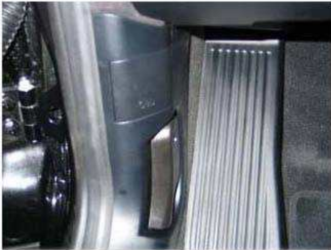
Fig. 18: Position DLC For X3 Models And Closed Design Cover Courtesy of BMW OF NORTH AMERICA, INC.
