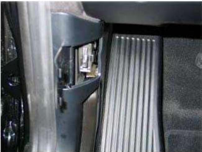
Fig. 19: Position DLC For X3 Models With Opened Design Cover And Closed Functional Cover Courtesy of BMW OF NORTH AMERICA, INC.
