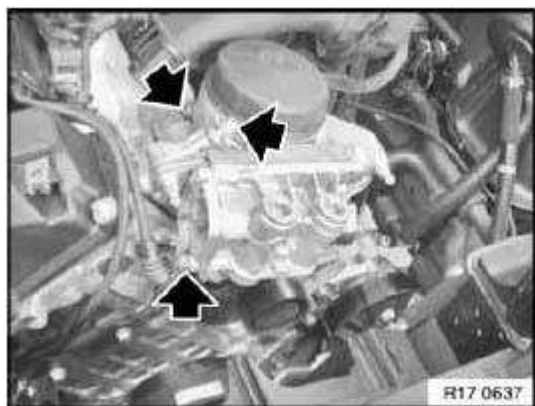
Fig. 60: Locating Mount Oil Filter Housing On Crankcase Courtesy of BMW OF NORTH AMERICA, INC.
