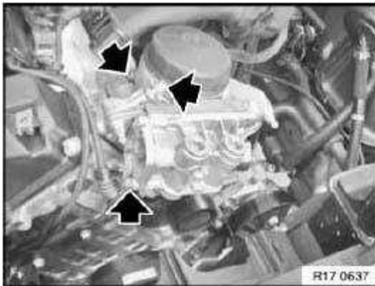
Fig. 2: Locating Mount Oil Filter Housing On Crankcase Courtesy of BMW OF NORTH AMERICA, INC.
