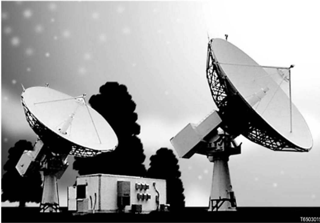
Fig. 14: Identifying SDARS Ground Transmitting Antenna Courtesy of BMW OF NORTH AMERICA, INC.
