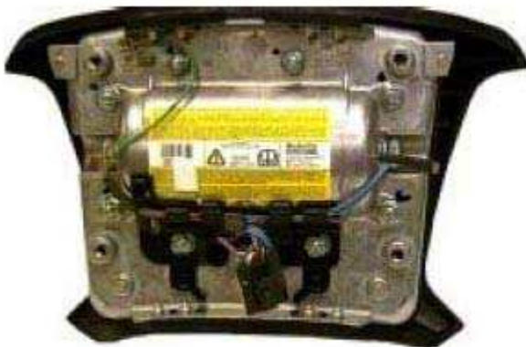
Fig. 10: Identifying Driver Side SMART Airbag System Courtesy of BMW OF NORTH AMERICA, INC.
