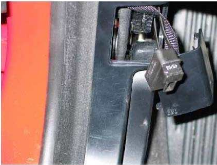
Fig. 23: Position DLC For 3 Series Models And Opened Design Cover / Opened Functional Cover Courtesy of BMW OF NORTH AMERICA, INC.
