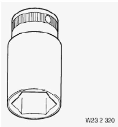
Fig. 82: Socket For Socket Wrench WAF 36 (23 2 320) Courtesy of BMW OF NORTH AMERICA, INC.
