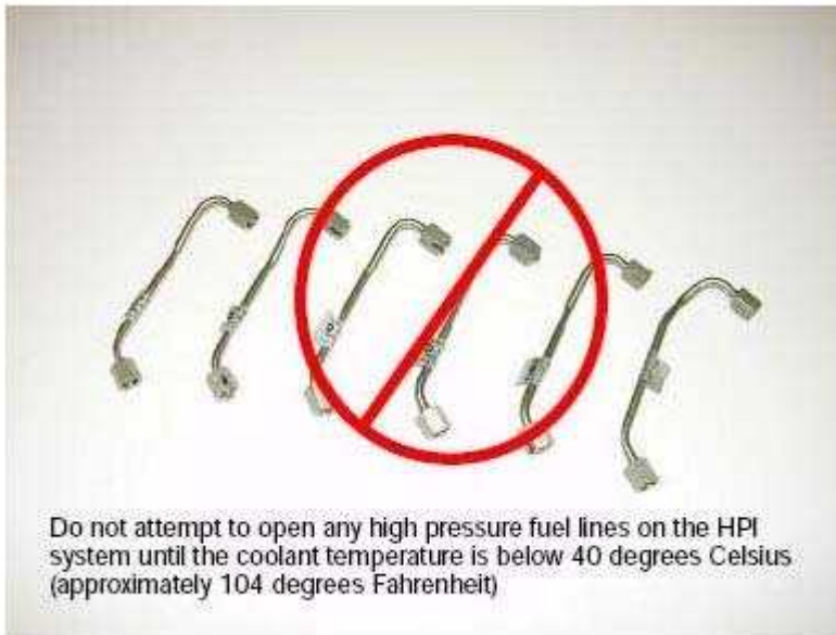
Fig. 58: Identifying High-Pressure Fuel Lines Courtesy of BMW OF NORTH AMERICA, INC.
