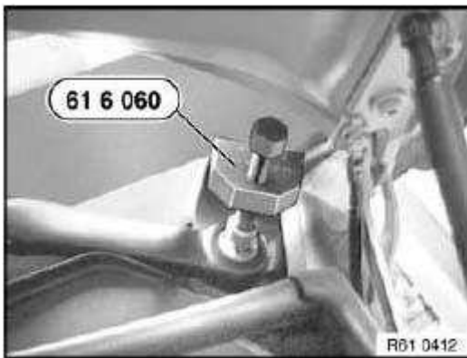
Fig. 218: Identifying Special Tool (61 6 060)
