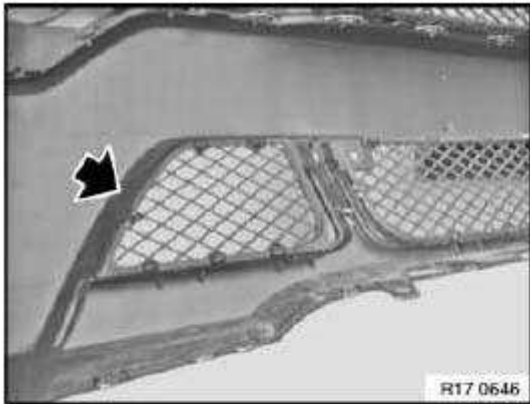
Fig. 69: Locating Bumper Trim With Grille Panel Courtesy of BMW OF NORTH AMERICA, INC.
