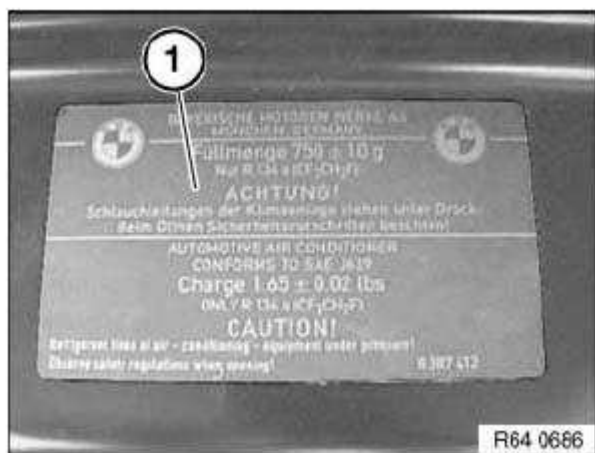
Fig. 55: Instructions For Filling A/C System Screen Courtesy of BMW OF NORTH AMERICA, INC.
