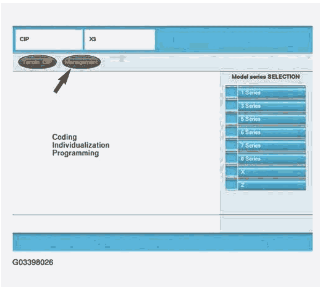
Fig. 172: Selecting "Management" From Main/Initial CIP Screen (1 Of 2) Courtesy of BMW OF NORTH AMERICA, INC.
