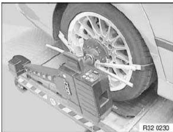
Fig. 10: Measuring Sensors With CCD Camera Courtesy of BMW OF NORTH AMERICA, INC.
