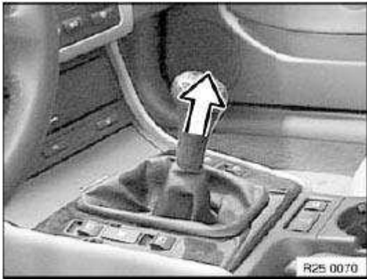
Fig. 2: Detaching Knob With Firm Tug Courtesy of BMW OF NORTH AMERICA, INC.
