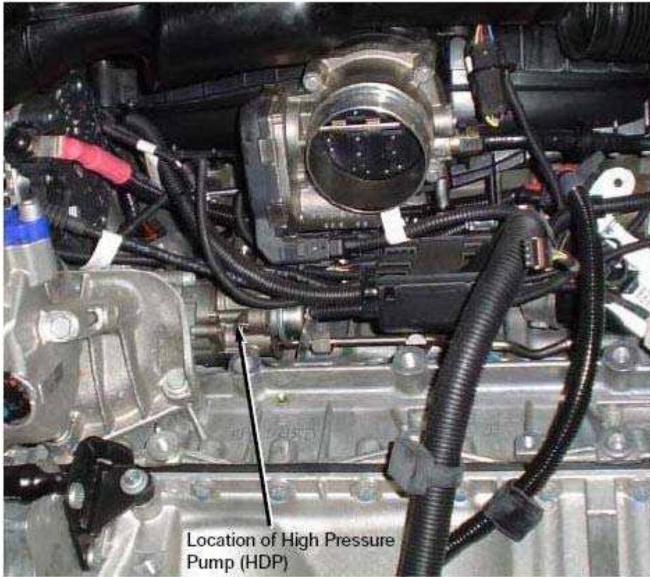
Fig. 55: Identifying High-Pressure Pump Location (HDP) Courtesy of BMW OF NORTH AMERICA, INC.
