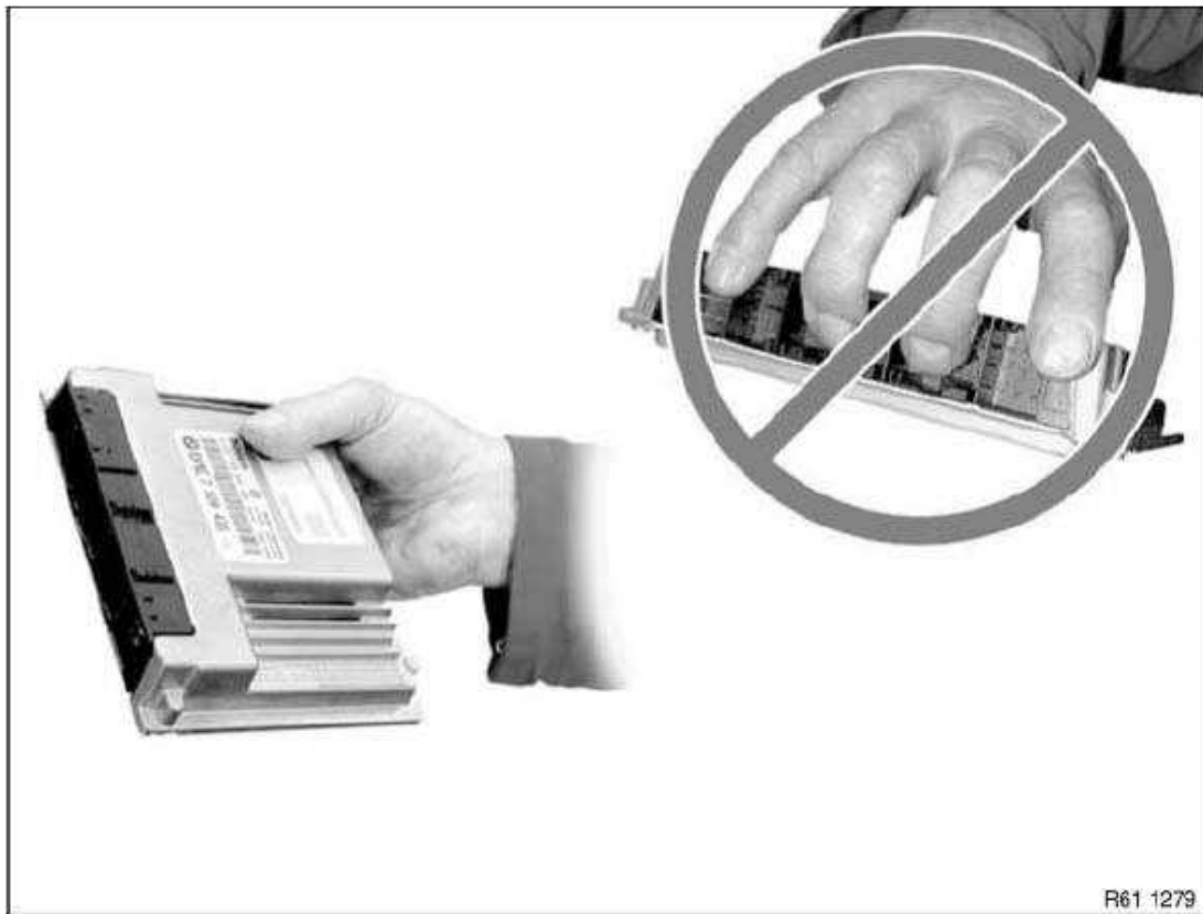
Fig. 186: Precaution For - Do Not Touch Pins Or Multi-Pin Connectors Directly Courtesy of BMW OF NORTH AMERICA, INC.
