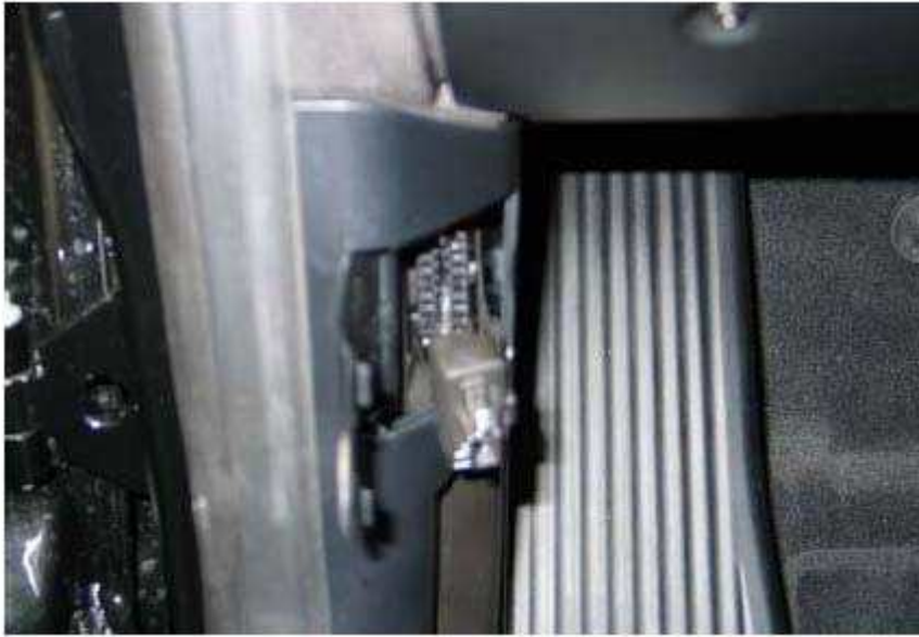
Fig. 20: Position DLC For X3 Models With Opened Design Cover And Opened Functional Cover Courtesy of BMW OF NORTH AMERICA, INC.
