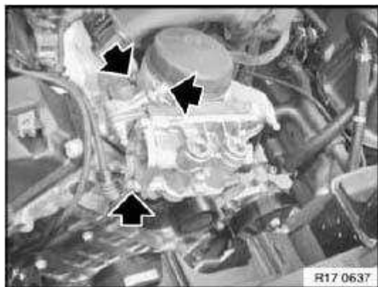
Fig. 32: Locating Mount Oil Filter Housing On Crankcase Courtesy of BMW OF NORTH AMERICA, INC.
