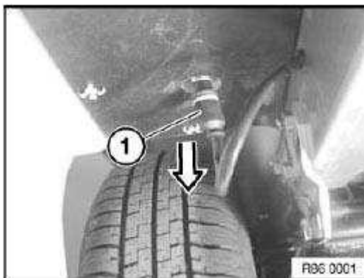
Fig. 106: Identifying Cable Tie, Grommet & Socket Courtesy of BMW OF NORTH AMERICA, INC.
