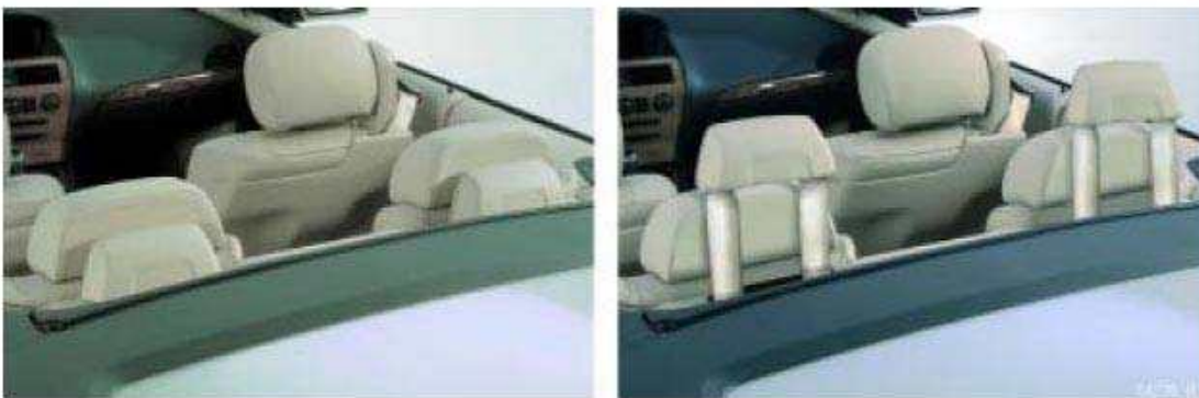
Fig. 24: Identifying Rollover Protection (RPS) Systems Courtesy of BMW OF NORTH AMERICA, INC.
