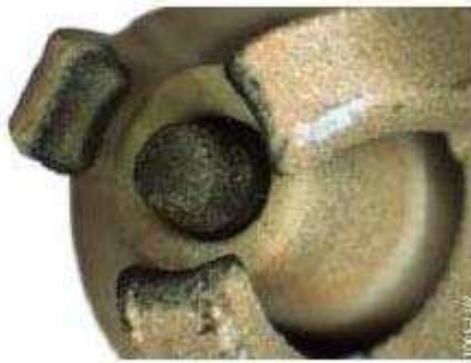
Spark plug showing normal wear pattern for high mileage
