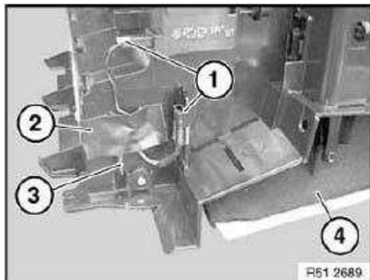
Fig. 224: Plug Connections, Cable And Glovebox Courtesy of BMW OF NORTH AMERICA, INC.
