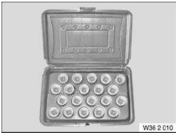
Fig. 11: Set Of BMW Wheel Bolt Adapters (36 2 010) Courtesy of BMW OF NORTH AMERICA, INC.
