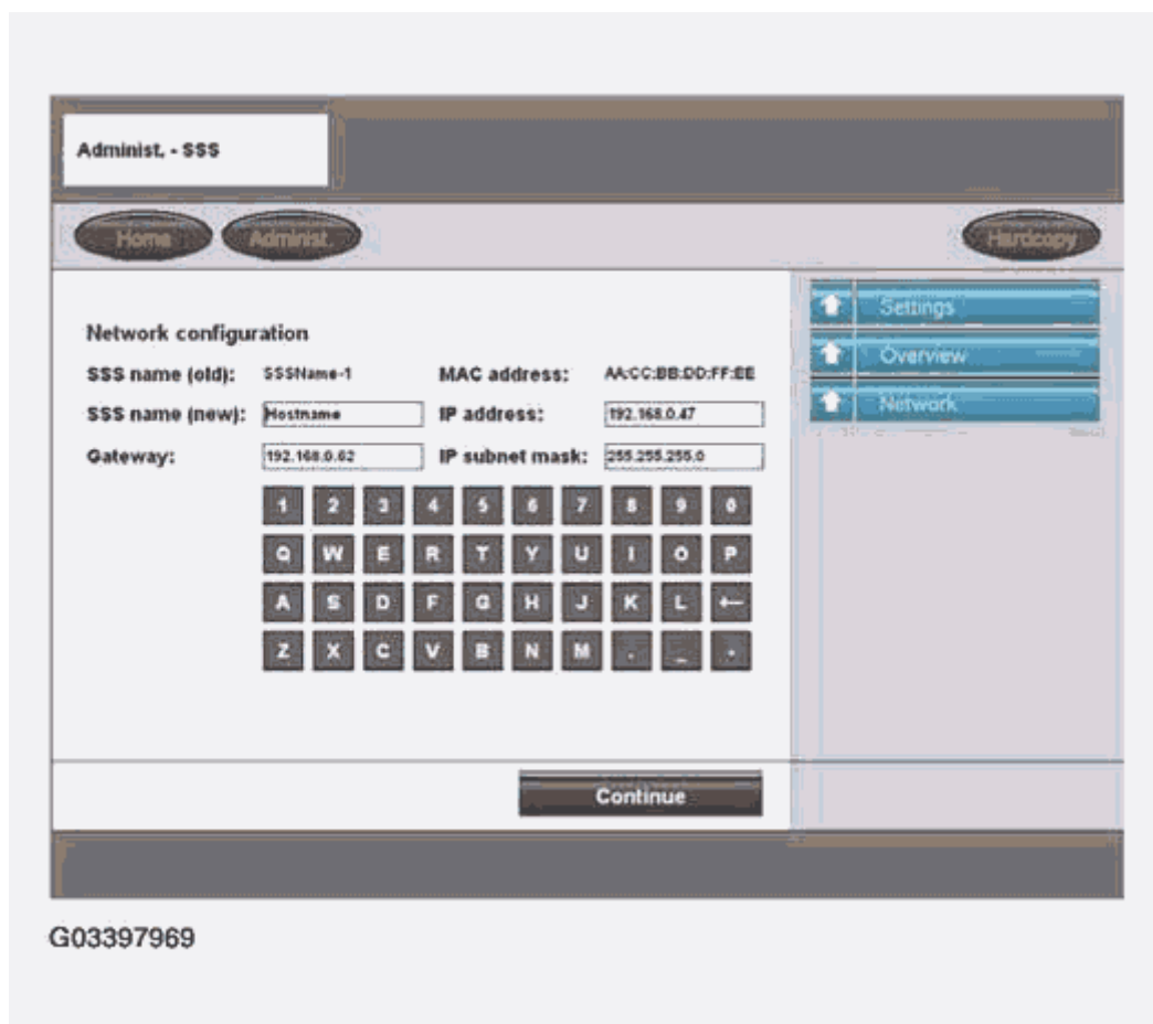
Fig. 115: Display Network Configuration Menu (1 Of 2) Courtesy of BMW OF NORTH AMERICA, INC.
