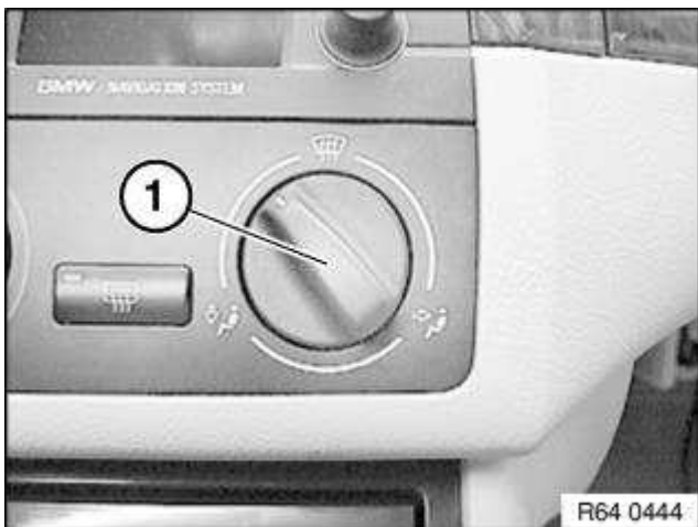
Fig. 33: Move Rotary Knob (1) Into Position Illustrated Courtesy of BMW OF NORTH AMERICA, INC.
