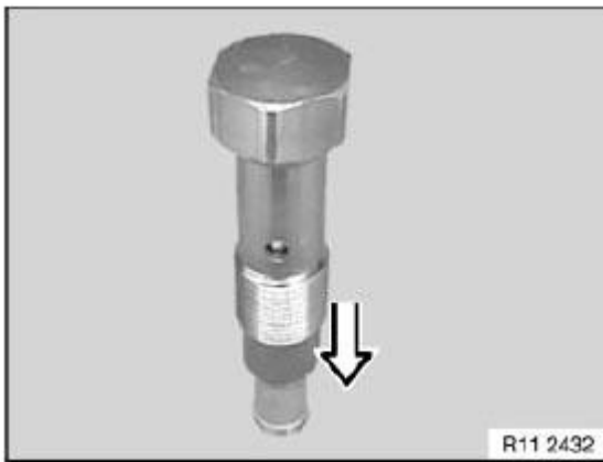
Fig. 245: Compressing Chain Tensioner On A Level Working Surface
