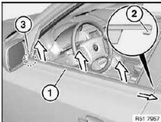
Fig. 271: Window Cavity Cover Strip, Guide And Door Mirror Courtesy of BMW OF NORTH AMERICA, INC.
