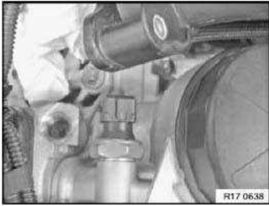
Fig. 3: Locating Mount Oil Pressure Switch On Filter Housing Courtesy of BMW OF NORTH AMERICA, INC.
