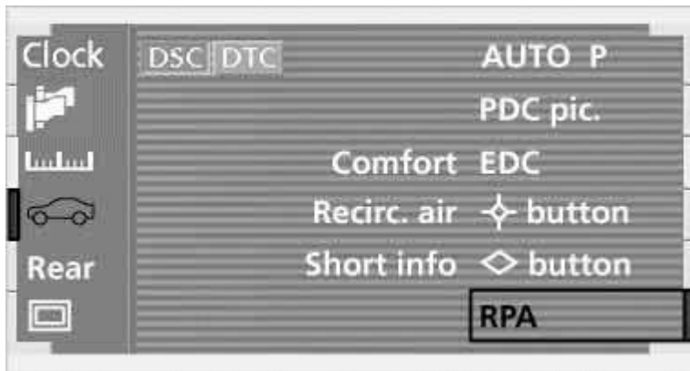
Fig. 13: Identifying TPM System Reinitialization Messages (1 Of 2) Courtesy of BMW OF NORTH AMERICA, INC.
