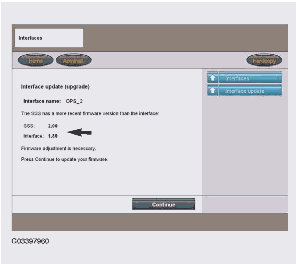
Fig. 106: Display Interface Update Information (1 Of 2) Courtesy of BMW OF NORTH AMERICA, INC.
